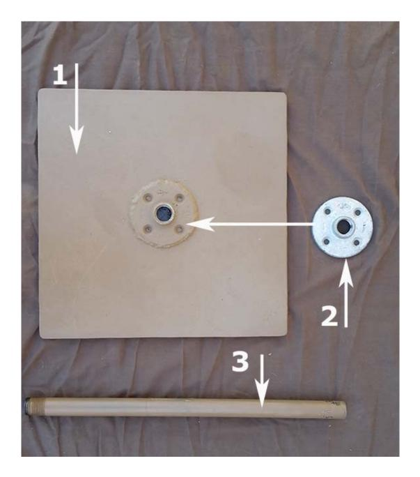
Larger pipe with a flange was used for this medium PVC pipe frame base. Either design will work. Pick your size.
